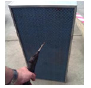
6. Inspect and blow with air the main dust control filter.
