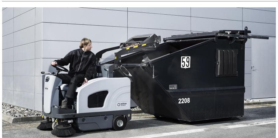
If the machine has been used until the Red light illuminates on the battery level indicator on the machine, a full recharge of the batteries (10-12 hours) will be required. Failure to carry out this this procedure may cause damage to the batteries. Charging the batteries after every use is recommended.
