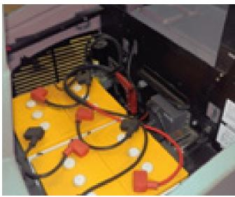
2. For the battery version check the battery voltage and charge if needed.
