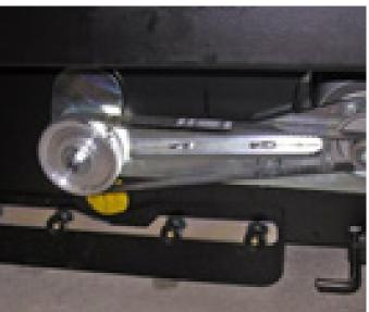
12. Check the main broom belt tension and general condition
