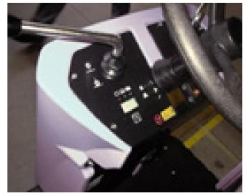
1. Check the diesel fuel tank level/LPG bottle/ Battery charge. In case refill/ change the LPG bottle.
