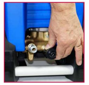
1. Remove water inlet coupling from machine.
