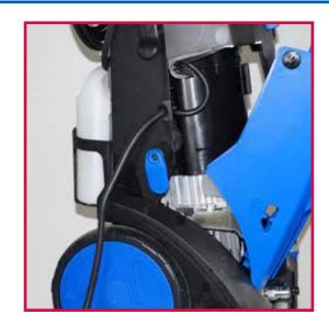
2. Remove front cabinet by turning 2 quarter turn screws at right and left top cabinet side.
