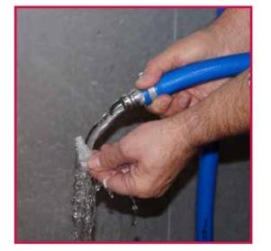
3. Rinse filter with running clean water / or compressed air.
