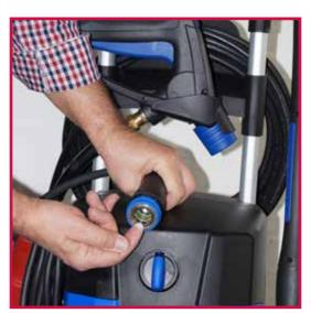
2. 3/8" hose quick coupling being greased. Use water resistant lubricant.
