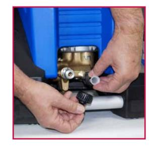
4. Reinstall water inlet filter and water inlet coupling.
