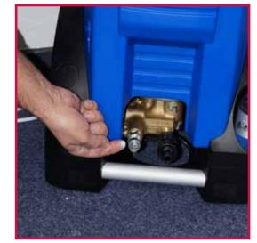
3. 3/8" High Pressure Nipple being greased. Use water resistant lubricant.
