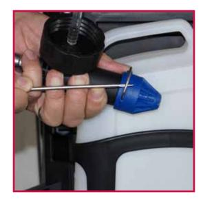
2. Use screwdriver to remove pin on FoamSprayer.
