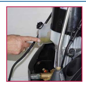
3. If neccessary refill oil to max. level point for the model in question.
