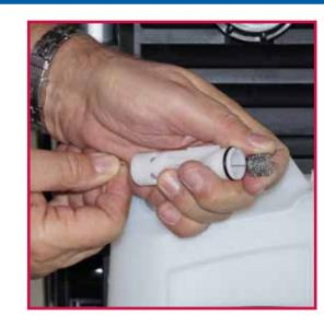
4. Use paper clip to push out the SS sponge and rinse with temperated water / compressed air. Repeat until clean.
